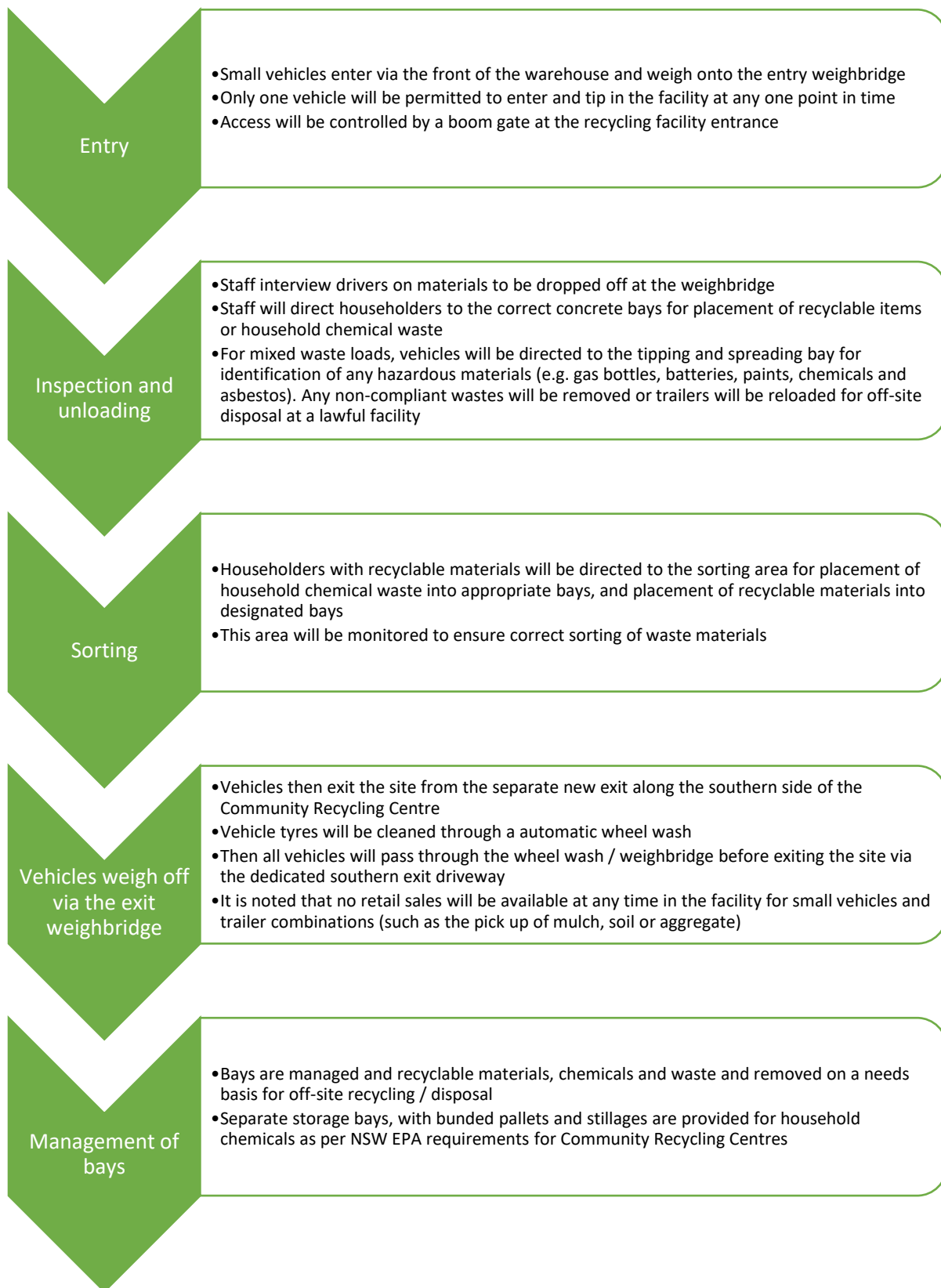
Figure 3.1. Process flow chart for the operation of the Community Recycling Centre – Small vehicles with clean-up waste, household chemical waste and recyclables.
