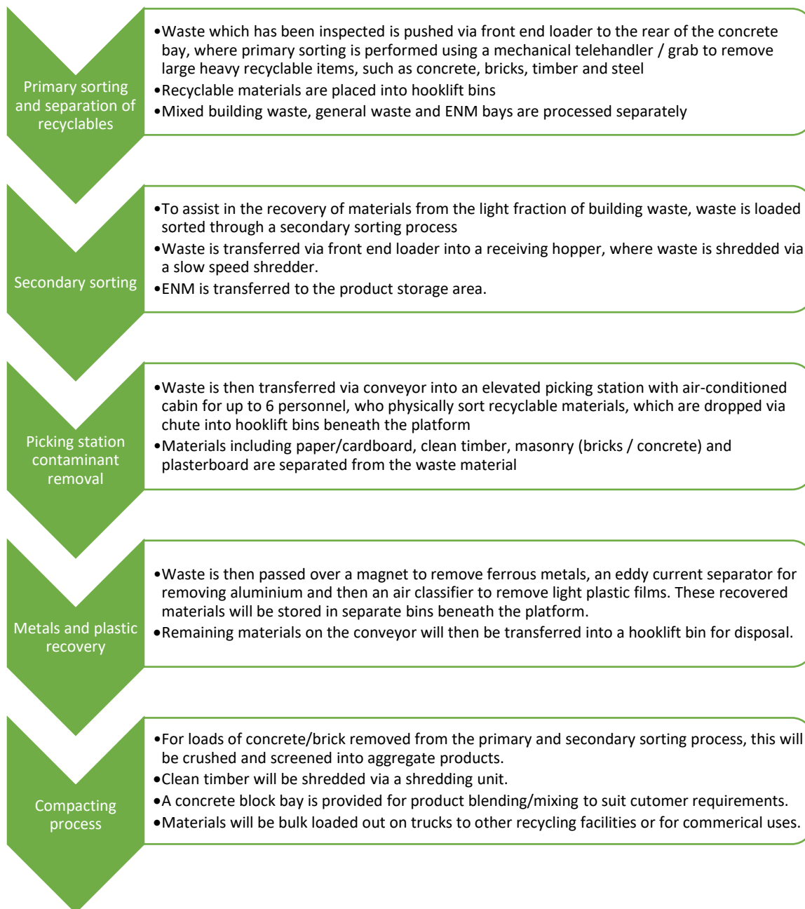
Figure 3.3. Process flow chart for the operation of the Processing Area.
