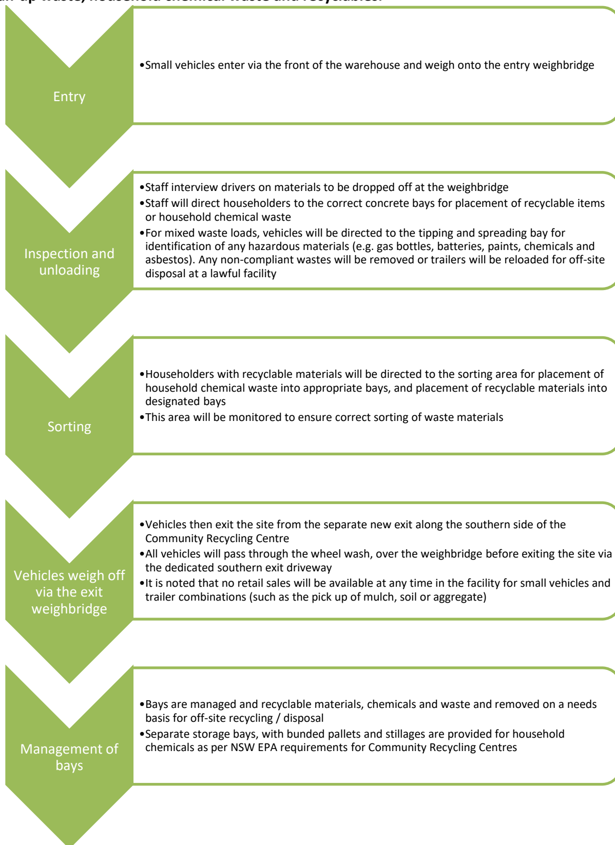
Figure 2.5. Process flow chart for the operation of the Community Recycling Centre – Small vehicles with clean-up waste, household chemical waste and recyclables.
