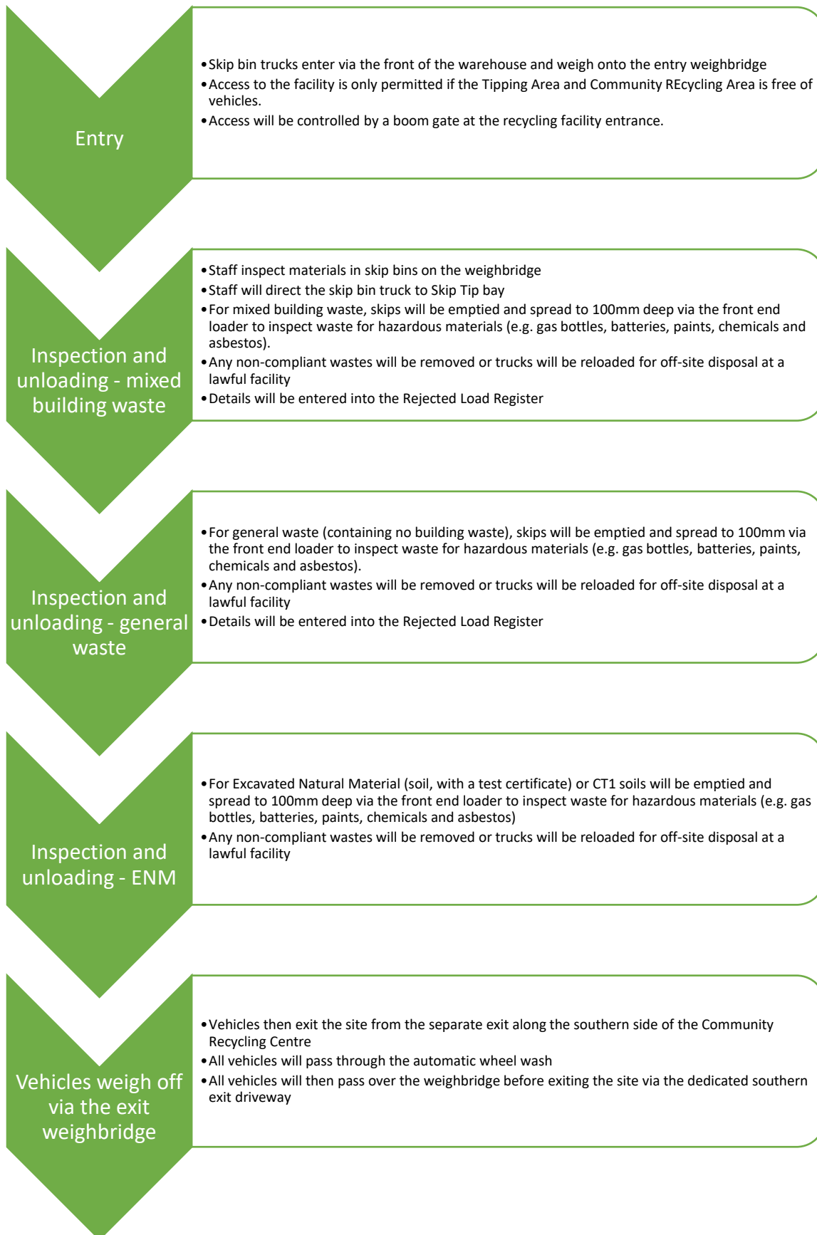
Figure 3.2. Process flow chart for the operation of the Tipping Area.
