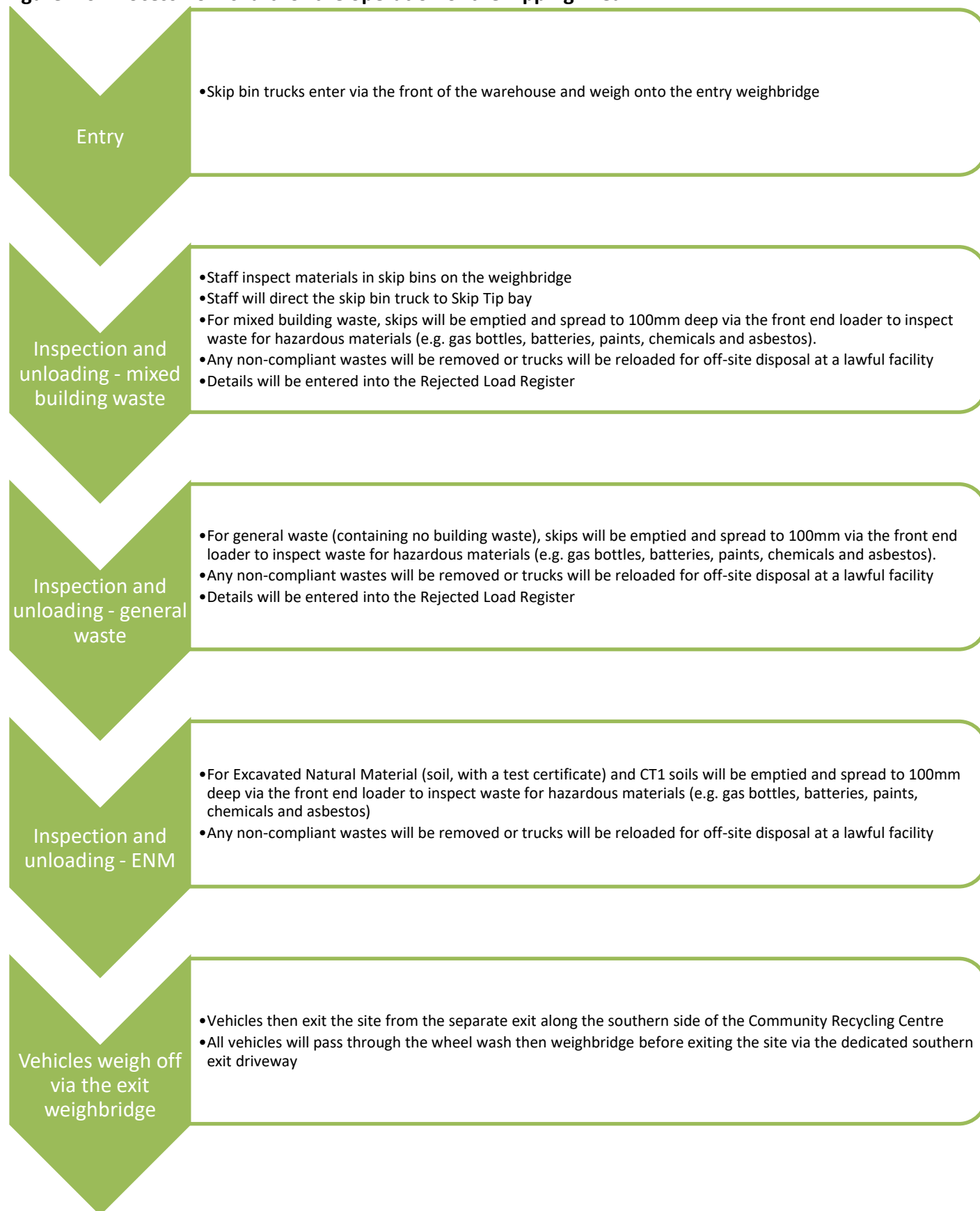
Figure 2.6. Process flow chart for the operation of the Tipping Area.
